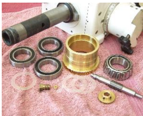
All of the components from the RA axis removed, cleaned and lubricated
