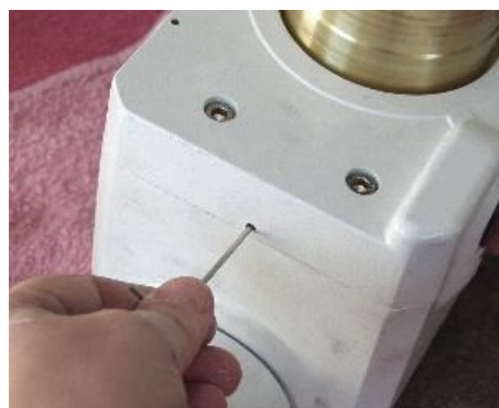
Tighten the lower set screw enough so that it is no longer proud of the casing.
