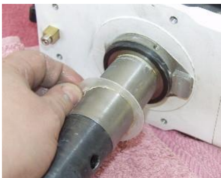
Beneath the RA worm gear will be another Teflon washer. Make sure this is removed and set aside and kept separate from all other washers.
