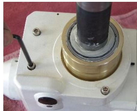
Tighten the cap headed screws down but not too tight. Allow some small movement to take place in the worm carrier.
