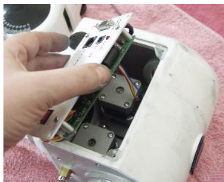
Gently pull the control panel away, revealing the motor control board. You can either disconnect the motors from the main board or leave alone and extract all of the motors and control board as one unit.
