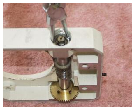
Remove the slotted nut from the worm carrier using circlip pliers, snipe nosed pliers, two small Allen keys or two fine tipped screwdrivers.
