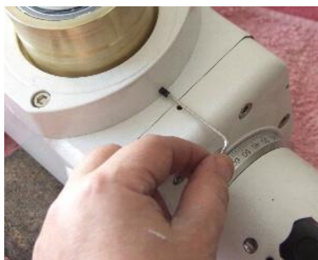
Tighten the upper set screw enough so that it is no longer proud of the casing.
