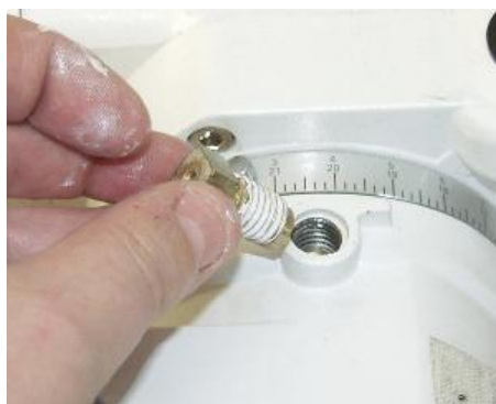
Apply some lithium grease to the RA clutch locking bolt and then replace the bolt. Screw this in until it is tight and the declination axis is locked.
