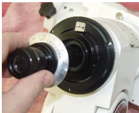
Replace the polar scope.
