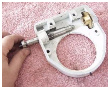
The worm will now simply pull free from the worm carrier.
