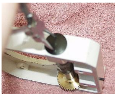
Remove the worm end-caps using some circlip pliers or snipe nosed pliers. You may also be able to remove these with two small Allen keys inserted. On this EQ6 these were VERY tight.
