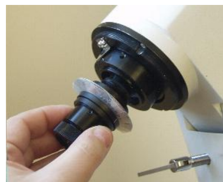
Once loosened simply unscrew the polar scope and place it somewhere safe.
