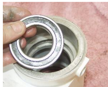
Remove the bearing from the mount base. This can be tapped out using a wooden pole and a mallet in the same way as the DEC housing main bearing shown in the DEC strip down module.
