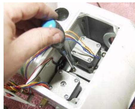
Remove the two screws from each motor and be careful not to lose the washers.
