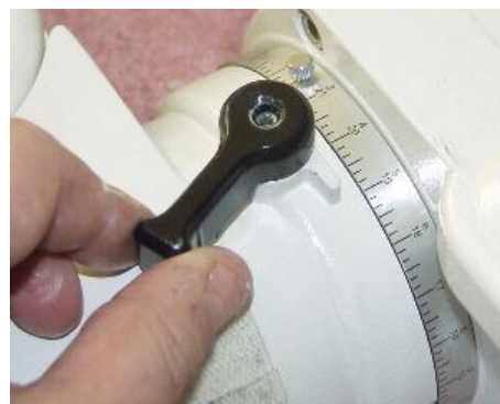
Replace the DEC clutch lever and test that you can both lock and free the DEC axis before replacing the screw and tightening it down.
