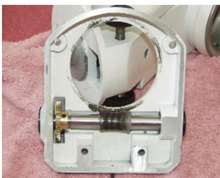
The picture above shows the worm carrier as removed from the mount. Note the position of the motor gear on the worm - it is not flat against the worms' widest point. This is correct.
