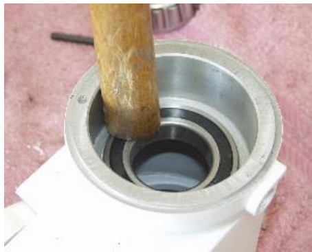
The mount base bearing may require to be tapped into place using a wooden driver. In this case the handle from an old hammer.
