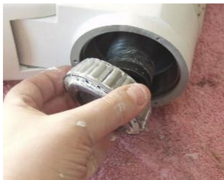
The mount base bearing may require to be tapped into place using a wooden driver. In this case the handle from an old hammer.
